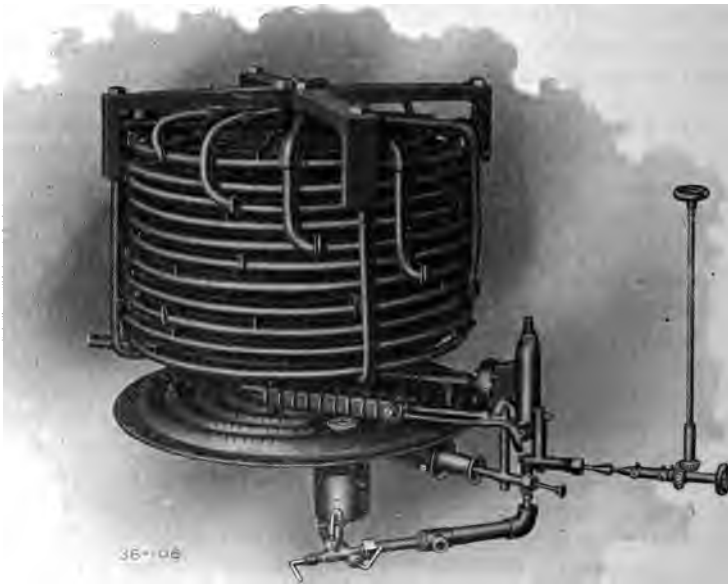
FIG. 347.—Diagram Illustrating Arrangement of the Vaporizing Coils of the White Flash Generator, Elevation. The water is fed into the centre of the top coil, flowing all around that coil and, in series , through every other coil in succession. It is "flashed" into steam somewhere above the lower coils, being taken off from the bottom one. The steam pipe rises to the top of the generator, as shown.
